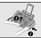
2 Gently pull the jammed paper out of the machine, making sure no torn pieces of paper remain in the print compartment or rollers.
